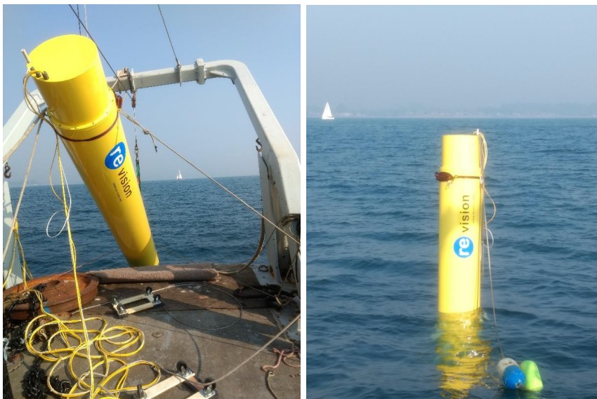
Illustration: 8kW In-Ocean Control Testing WEC Unit
